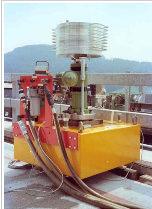
Fig 4: Servo-hydraulic shaker producing a 5 kN vertical force amplitude for 2.3 < f < 100 Hz (left). 500 kg mass are fixed to the piston rod of a cylinder with a \pm 50 mm stroke. The 40 l/min (280 bar) hydraulic power pack and associated air-cooler used to drive this cylinder are shown above.
