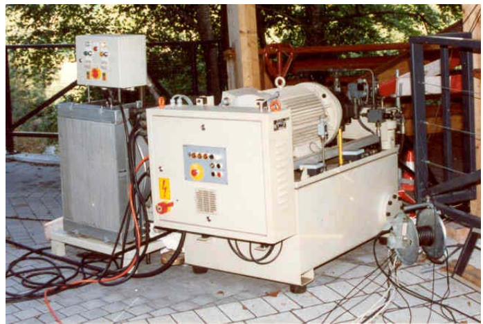
Fig 4: Servo-hydraulic shaker producing a 5 kN vertical force amplitude for 2.3 < f < 100 Hz (left). 500 kg mass are fixed to the piston rod of a cylinder with a \pm 50 mm stroke. The 40 l/min (280 bar) hydraulic power pack and associated air-cooler used to drive this cylinder are shown above.
