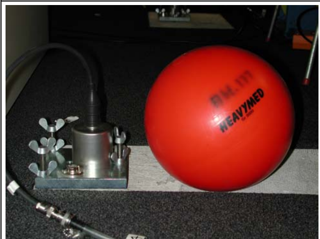
Fig. 34: Accelerometer and medical ball. The sensors were placed on the concrete without fixation but after removal of the carpet.
